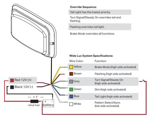
**Step 1**: In order to activate the unit, extend the red, 12V+ wire to the 12V+ post of the vehicle's battery. Extend the black, 12V-wire to the ground post of the vehicle's battery.
